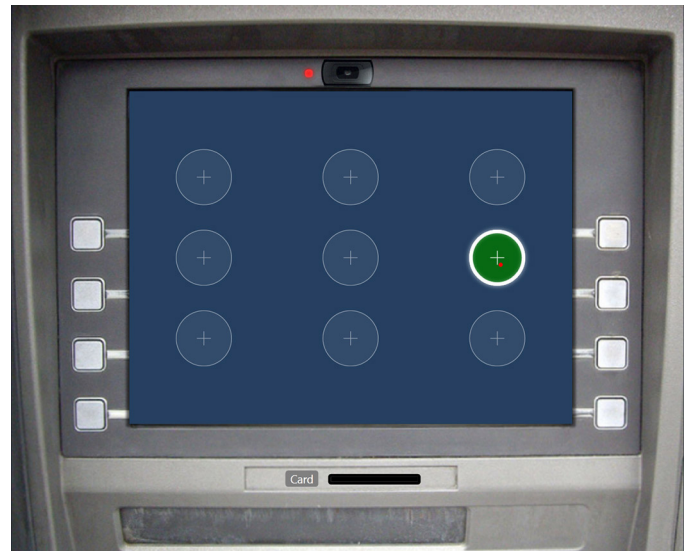
Figure 1. Users activate each circle using their gaze, while the eye tracker records eye movement data for authentication.
