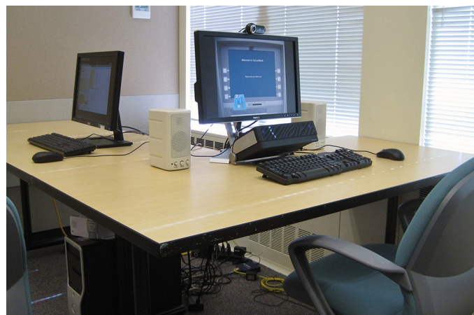
Figure 2. The eye tracker is positioned beneath the display in this automated teller machine authentication interface running on a computer.
